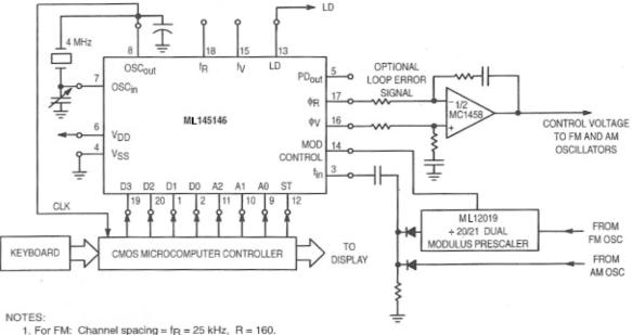
For AM: Channel spacing =  $f_R = 25$  kHz, R = 160. For AM: Channel spacing =  $f_R = 1$  kHz, R = 4000.
