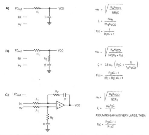
NOTE: Sometimes R1 is split into two series resistors, each R1 + 2. A capacitor CC is then placed from the midpoint to ground to further filter  $\phi_V$  and  $\phi_P$ . The value of C<sub>C</sub> should be such that the corner frequency of this network does not significantly affect  $\omega_n$ .
