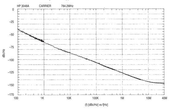
Figure 12. Typical Phase Noise Plot, 750 MHz Tank
