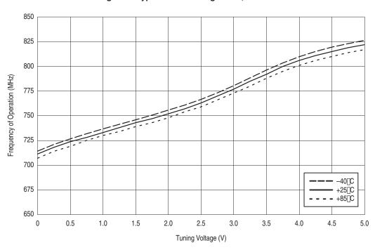
Figure 4. Typical VCO Tuning Curve, 750 MHz Tank
