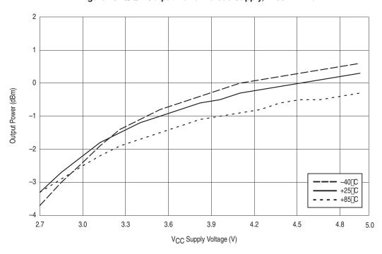
Figure 10. Q/QB Output Power versus Supply, 1200 MHz Tank
