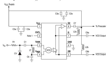
Figure 2. ML12149 Typical External Component Connections
